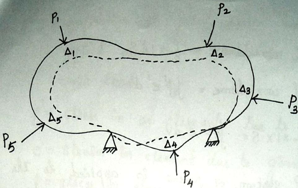
A body subjected to load and deformed shape.
