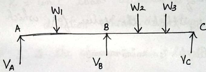
Figure shows a continuous beam. If the reaction at A is  $X$ , then the conditions of equilibrium are not sufficient to find the value of  $X$ . For instance assuming any value of  $X$ , the reactions  $V_B$  &  $V_C$  can be determined. Hence with infinite values of  $X$  with corresponding values of  $V_B$  &  $V_C$  along with the given loads, satisfy the conditions of equilibrium.
