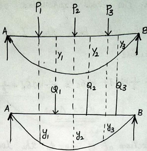
Let  $W_e$  = External work done on the structure when the system of forces  $P_1, P_2, P_3$  is applied
