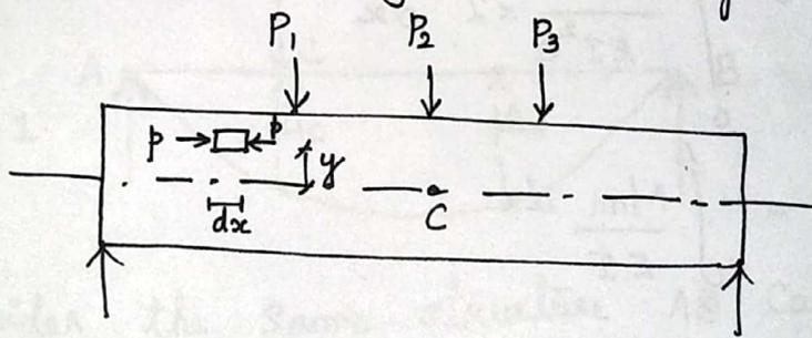
The stress in the element at a distance  $y$  from NA
